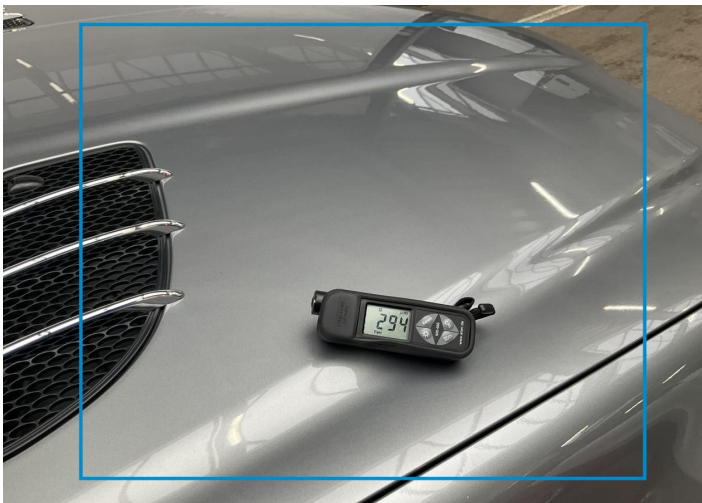
8. Hood Paint / Poor Previous Repair -
