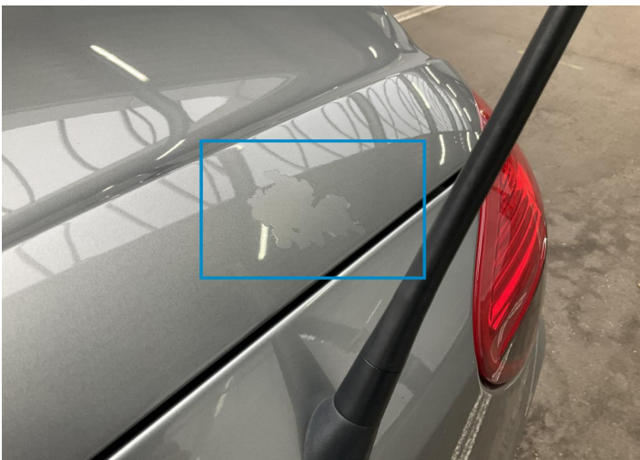
24. Tailgate Paint / Poor Previous Repair -
