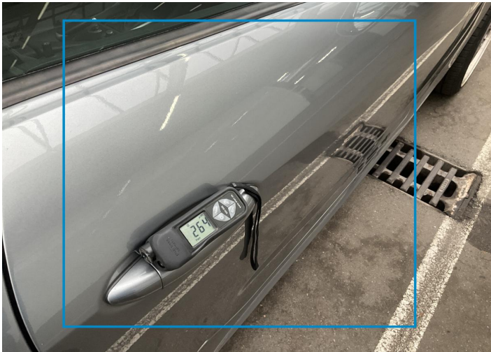
10. Door / Front Right Paint / Poor Previous Repair -
