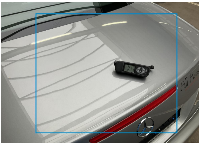
11. Tailgate Paint / Poor Previous Repair -
