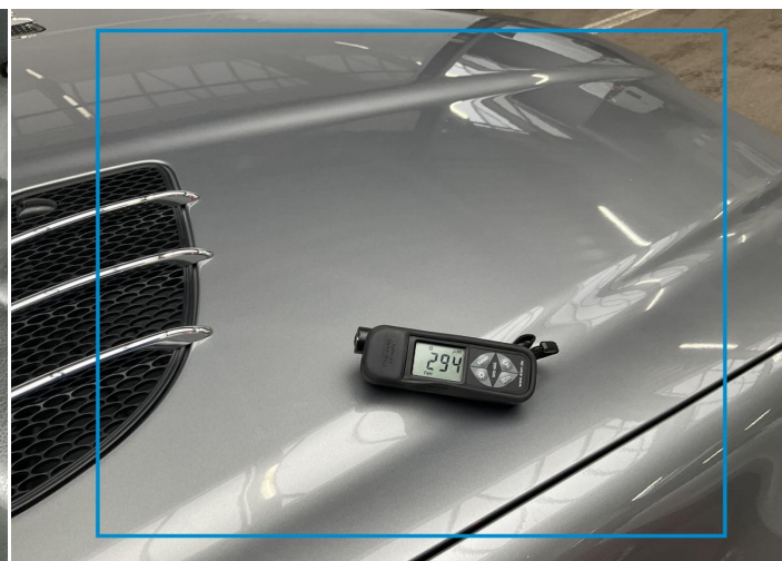
8. Hood Paint / Poor Previous Repair -
