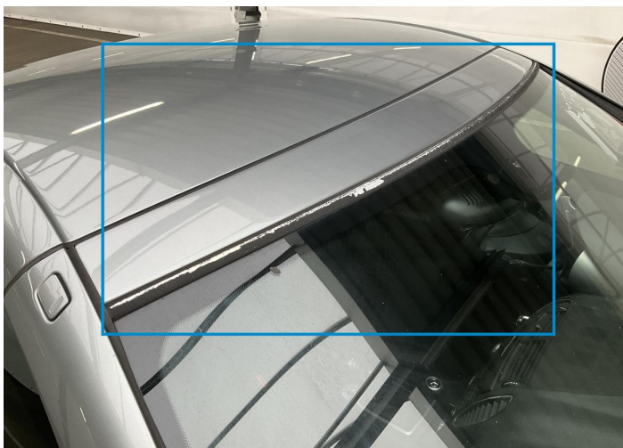
9. Roof Molding / Right Paint / Scratch / Scuff -
