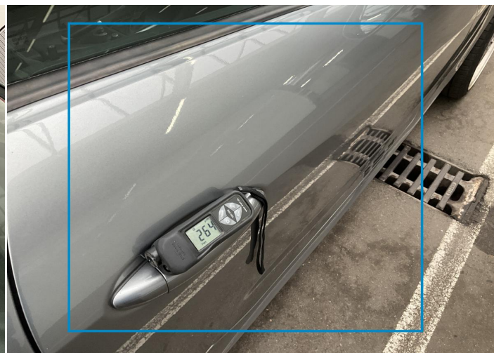
10. Door / Front Right Paint / Poor Previous Repair -
