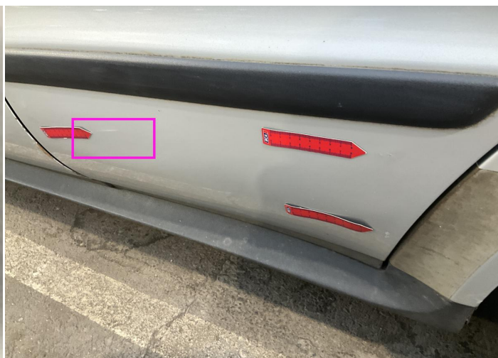
20. Door / Back Left Paint / Scratch / Scuff -
