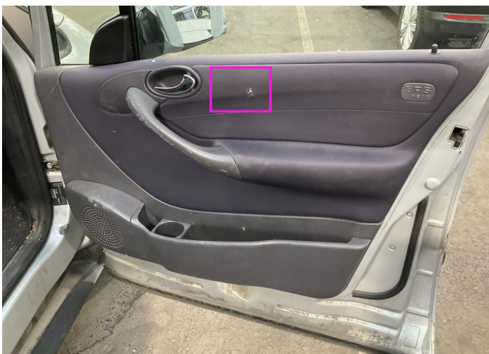
6. Panel Filling / Front Right Interior / Holed -
