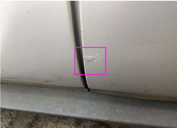
37. Door / Front Right Paint / Corrosion -
