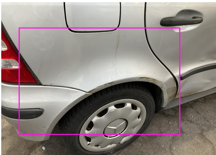
33. Side Panel / Back Right Paint / Corrosion -
