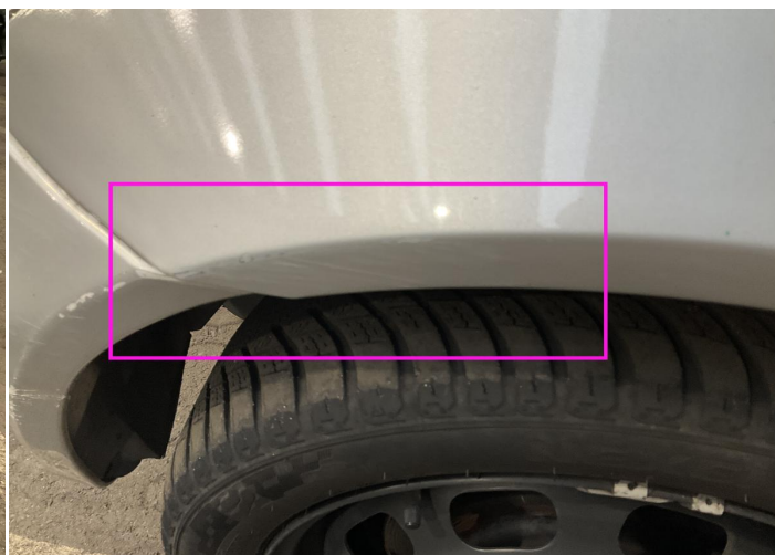
14. Fender / Front Left Paint / Scratch / Scuff -
