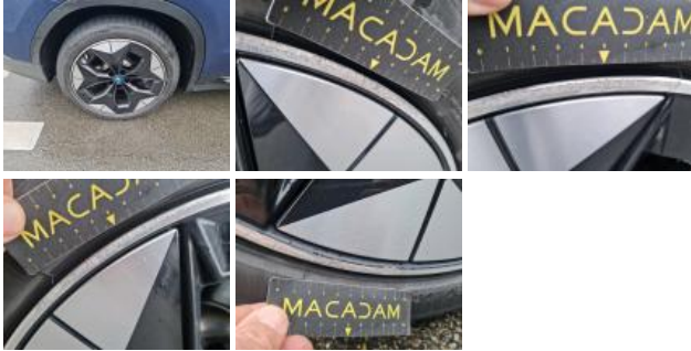
Alloy rim FR polished, Scratch(es), Repair and paint (complete)
