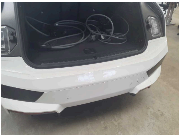
Damage #7: Rear bumper: Rear bumper - Dent / paintcoat dama... - Repair and paint
