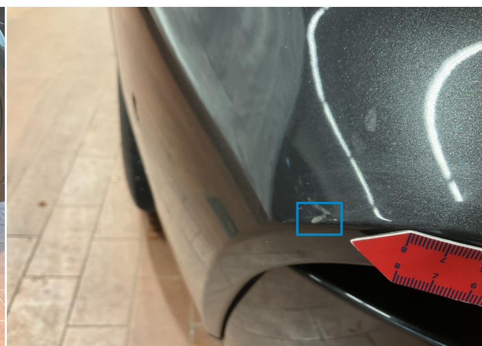
4. Bumper / Back Paint / Stone Chip -
