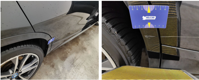
Wing Rear Right / Trim / Replace-scratch + dent
