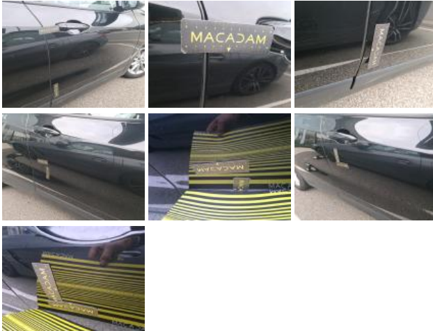
Outside rear-view mirror housing R, Scratch(es), Acceptable
