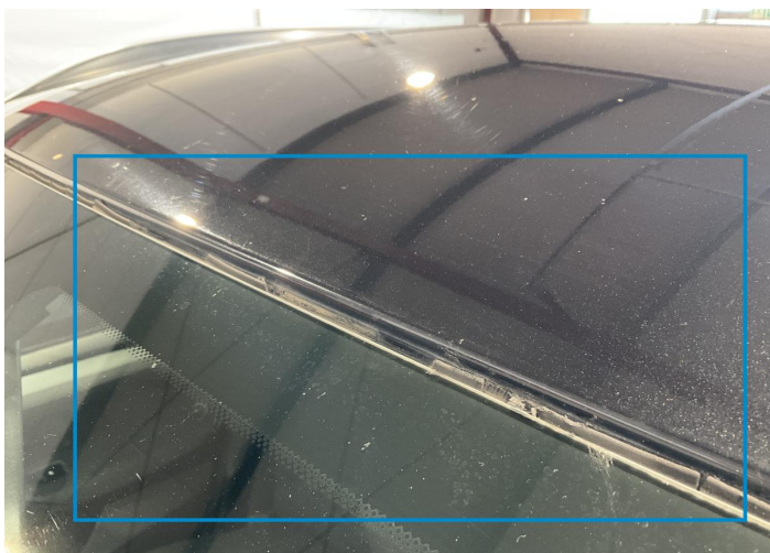
1. Windshield Joint / Front Bodywork / Breakage / Crack -
