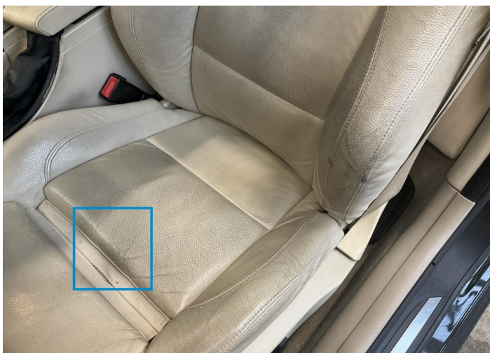
11. Seat / Front Left Interior / Ripped -
