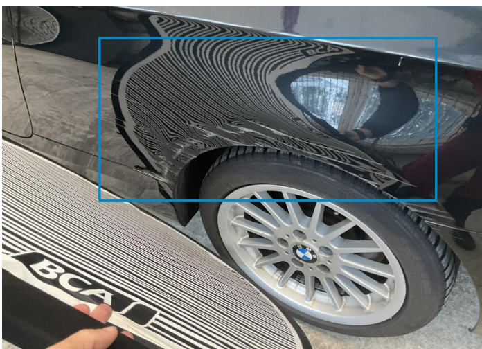
12. Fender / Back Left Bodywork / Dent / Dent -
