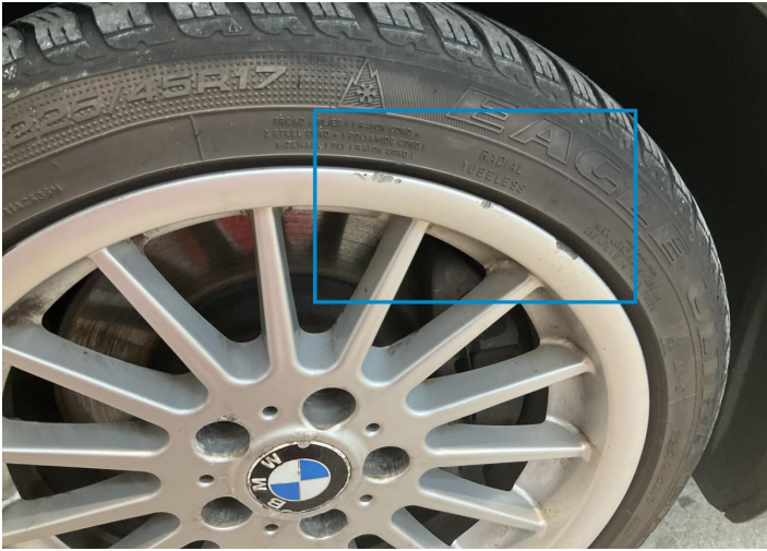
6. Rim / Front Left Out of Bodywork / Scratch -
