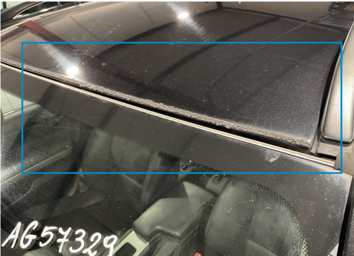
15. Windshield Joint / Front Bodywork / Breakage / Crack -
