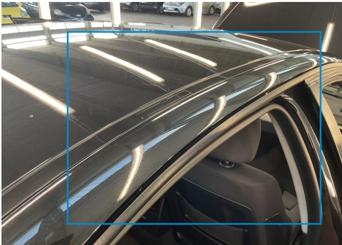
18. Pillar / Front Right Bodywork / Poor Previous Repair - 0.00
