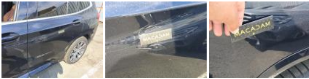
Wing RL, Scratch(es), Repair and paint (complete)
