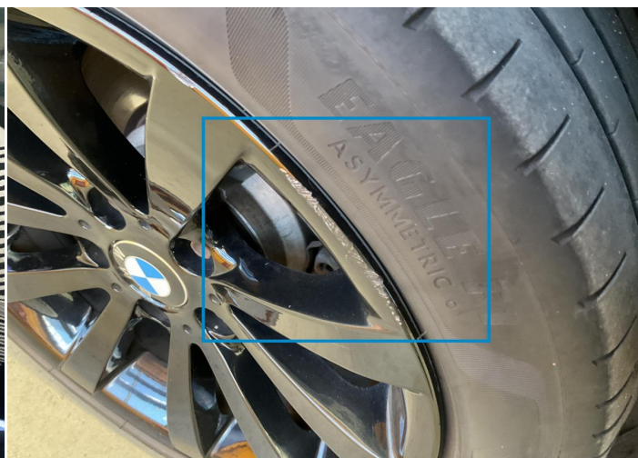
2. Rim / Front Left Out of Bodywork / Scratch -
