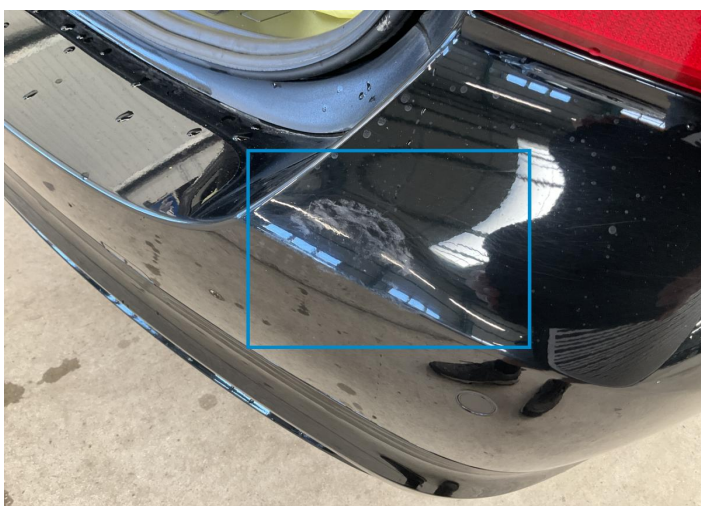
3. Bumper / Back Paint / Chemical Damage -
