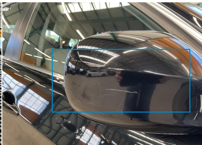
6. Mirror Shell / Front Right Paint / Scratch / Scuff -
