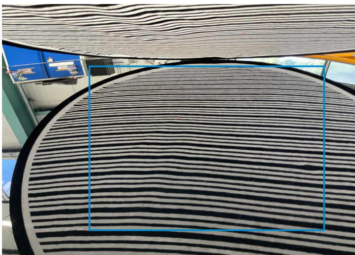
5. Roof Bodywork / Dent / Dent -
