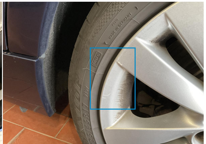
6. Rim / Back Left Paint / Stone Chip -
