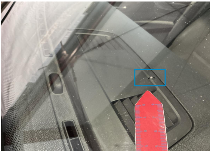
1. Windshield / Front Glass Break / Impact -
