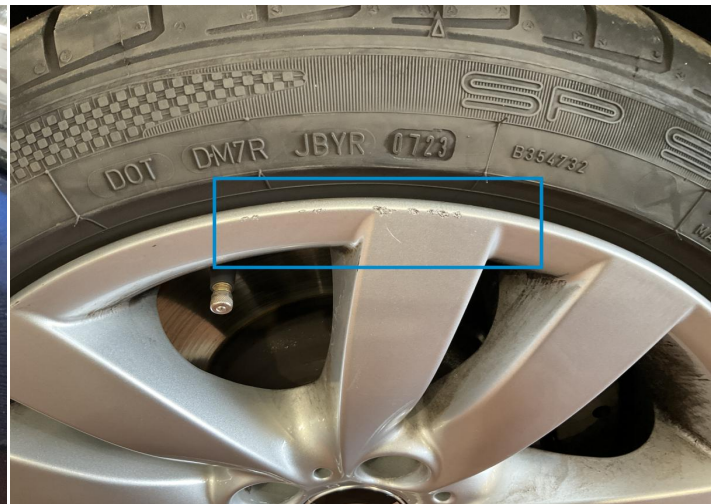
4. Rim / Front Left Paint / Stone Chip -
