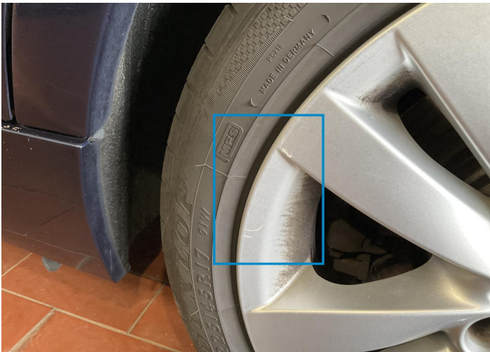
6. Rim / Back Left Paint / Stone Chip -
