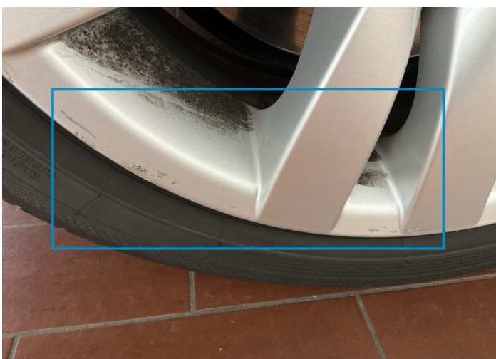
8. Rim / Back Right Out of Bodywork / Scratch -
