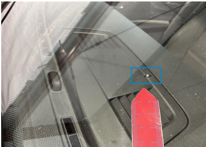
1. Windshield / Front Glass Break / Impact -
