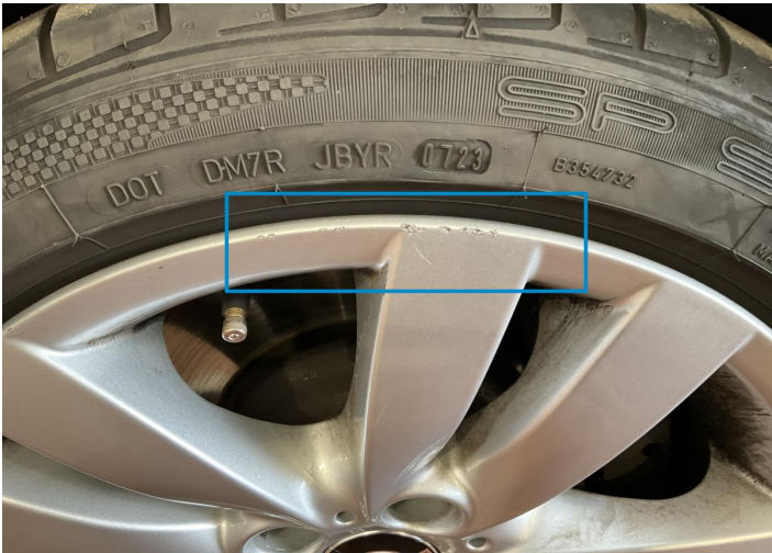
4. Rim / Front Left Paint / Stone Chip -
