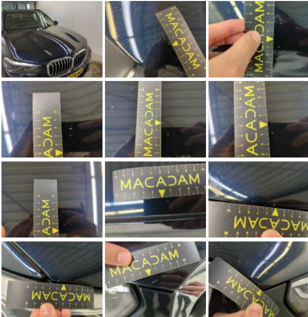
Bumper F, Scratch(es), Repair and paint (complete)
