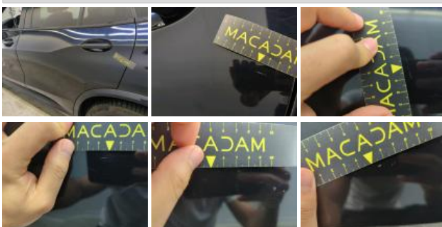
Door RL, Scratch(es), Repair and paint (complete)
