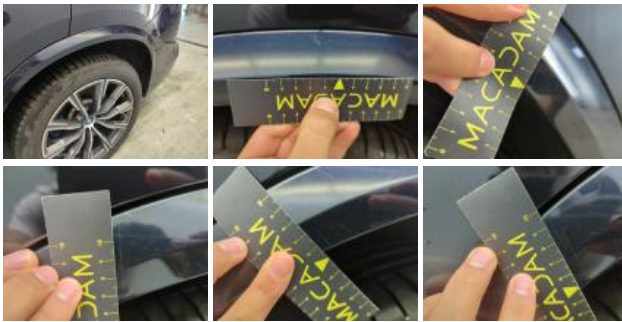
Outer sill L, Scratch(es), Repair and paint (complete)
