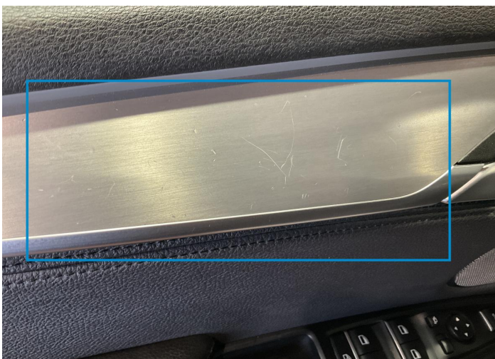
6. Panel Filling / Front Left Interior / Scratched -
