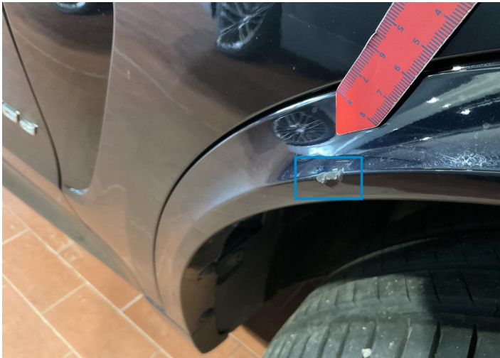
13. Wing Expander / Front Right Paint / Stone Chip -
