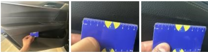
Door panel RR, Tear, Smart repair
