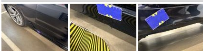
Outer sill L, Deformed / Strained, Replace and paint
