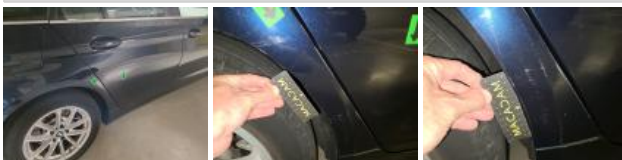
Door RR, Scratch(es), Repair and paint (complete)
