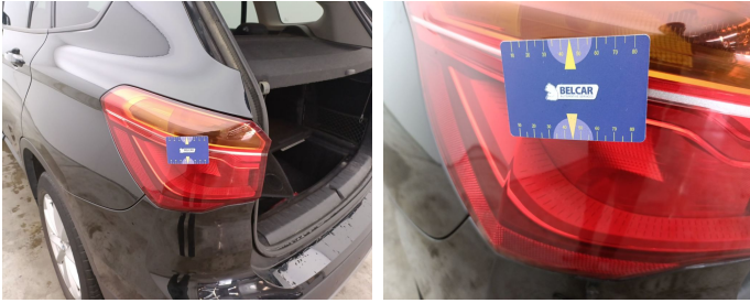
Light / Rear left / Replace-scratch
