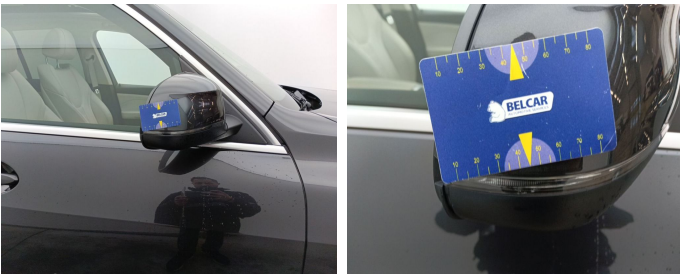
Side View Mirror Right / Direction Indicator / Replace-scratch
