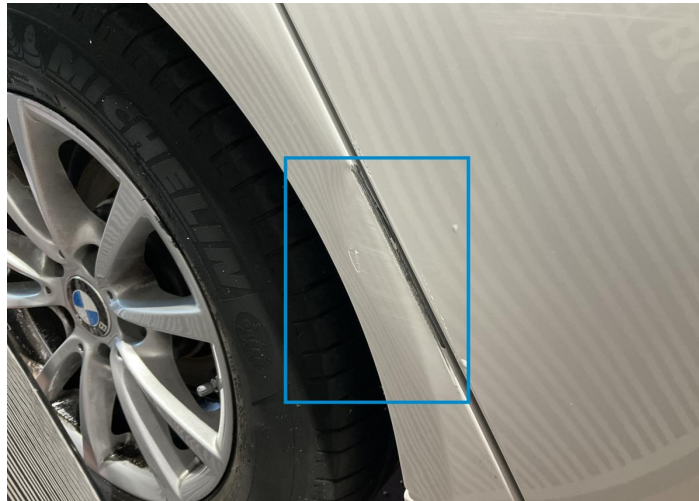
7. Side Panel / Back Right Bodywork / Dent / Dent -
