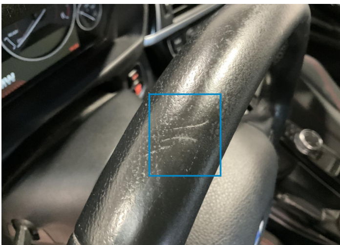
2. Steering Wheel / Front Interior / Scratched -
