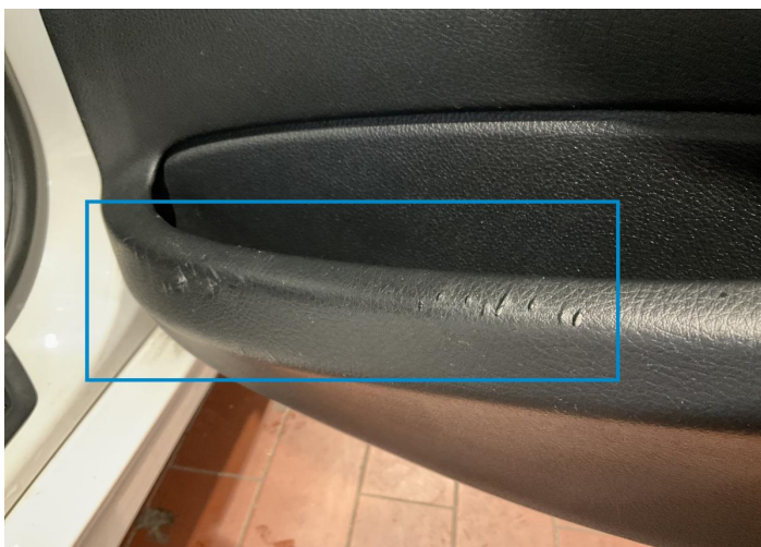
1. Panel Filling / Back Right Interior / Scratched -
