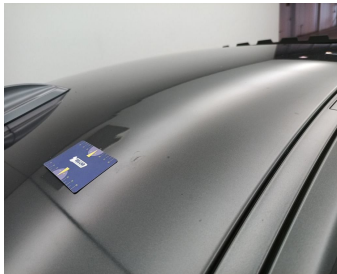
Wing Rear Right // Smart Repair Medium-dent
