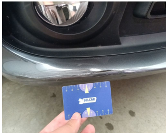
Bumper Front // Replace & Painting-cracked
