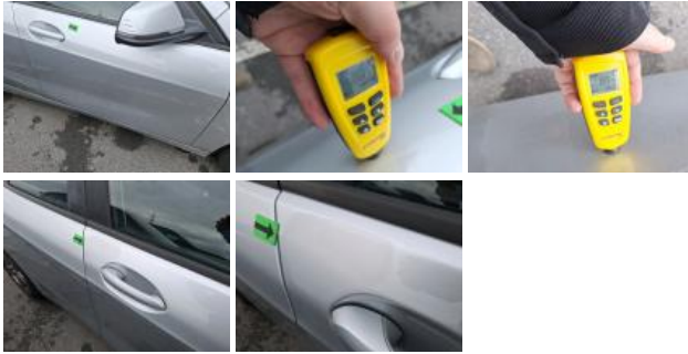
Wing FR, Repaired, Check
