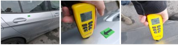
Door FR, Repaired, Polish
