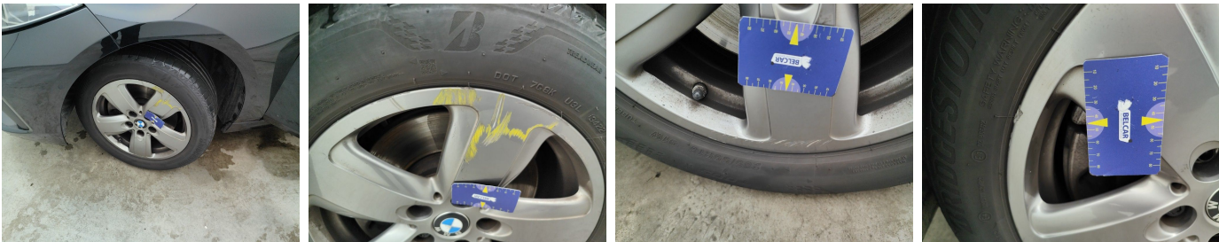
Wheel Alloy Front Left // Repair-scratch
