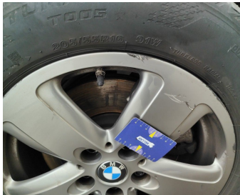
Wheel Alloy Front Right // Repair-scratch
