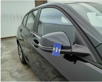
Side View Mirror Right / Direction Indicator / Replace-cracked
