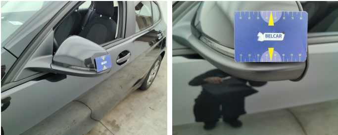
Side View Mirror Left // Replace Not Painted-scratch
