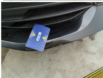
Bumper Front // Repair & Painting-scratch + dent
