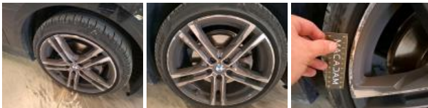
Tyre FR, Tear, Replace
