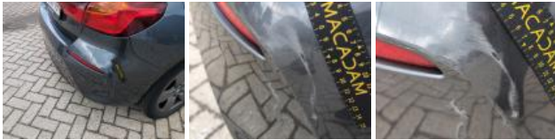
Wing RR, Scratch(es), Repair and paint (complete)
