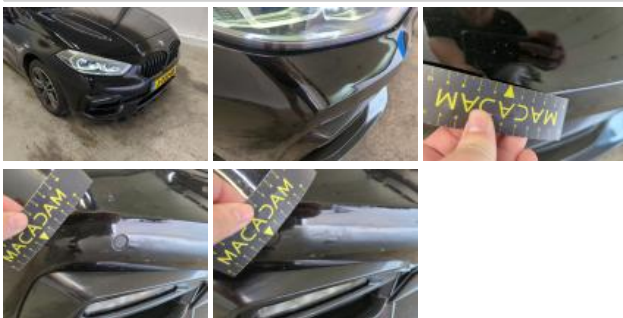
Grille frame, Scratch(es), Smart repair
