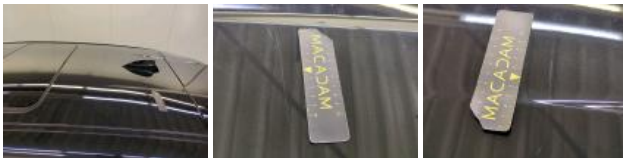
Roof, Scratch(es), Repair and paint (complete)
