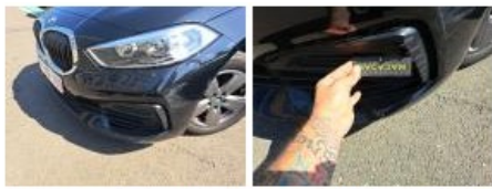
Bumper F, Scratch(es), Repair and paint (complete)
