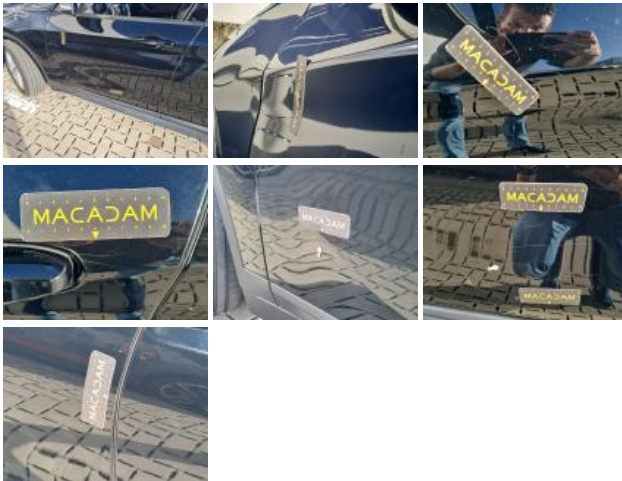
Roof pillar L, Scratch(es), Acceptable
