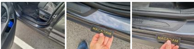
Internal boot lining R, Scratch(es), Acceptable
