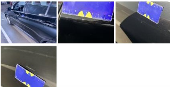
Roof pillar L, Dent(s), Paintless dent repair
