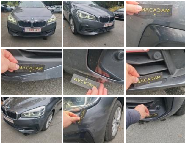
Bumper moulding F, Scratch(es), Replace
