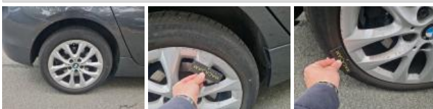
Alloy rim RR, Deformed / Strained, Replace
