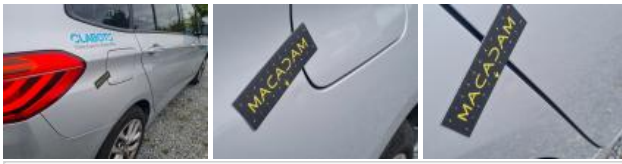
Sill trim R, Scratch(es), Repair and paint (complete)
