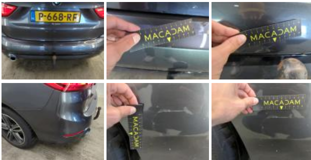
Bumper moulding R, Scratch(es), Replace and paint
