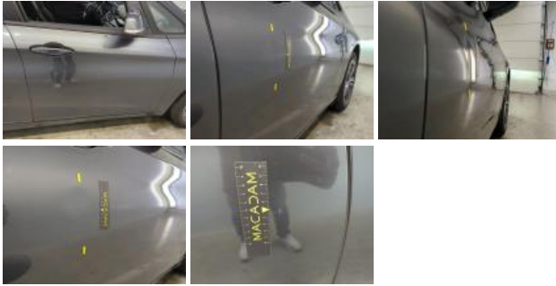
Door RR, Scratch(es), Repair and paint (partial)
