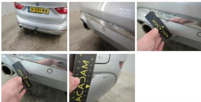
Bumper moulding R, Dent(s) and scratch(es), Replace
