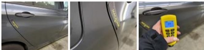
Door FR, Scratch(es), Repair and paint (complete)
