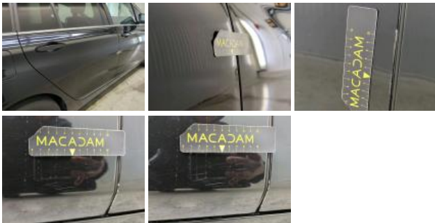
Door FR, Scratch(es), Repair and paint (complete)
