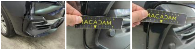
Bonnet, Chemical polution, Repair and paint (complete)
