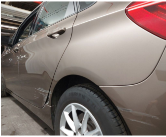
Wing Rear Left // Repair & Painting-scratch + dent
