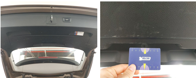
Trunk Lid Interior Coating / Complete Panel / Replace-scratch
