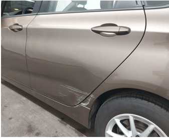
Door Rear Left // Repair & Painting-scratch + dent
