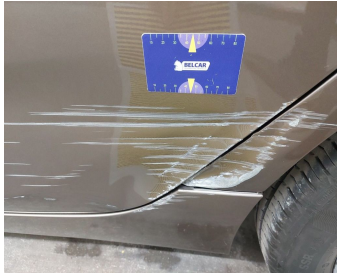
Door Rear Left // Repair & Painting-scratch + dent
