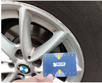
Wheel Alloy Rear Right // Repair-scratch
