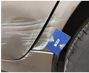
Wing Rear Left // Repair & Painting-scratch + dent
