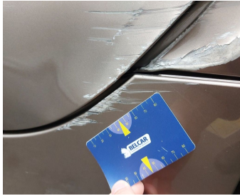
Door Rear Left // Repair & Painting-scratch + dent
