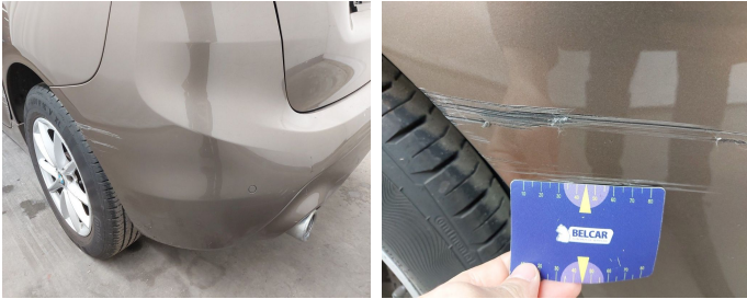
Bumper Rear // Smart Repair Medium-scratch
