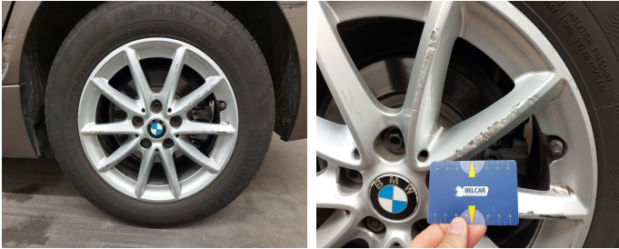
Wheel Alloy Rear Left // Repair-scratch
