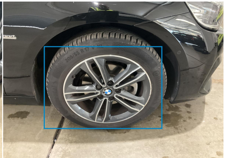
4. Rim / Front Right Out of Bodywork / Scratch -
