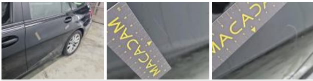
Door FL, Scratch(es), Repair and paint (complete)
