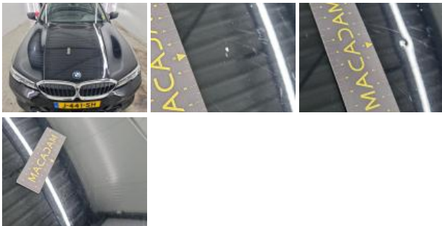
Door FR, Scratch(es), Repair and paint (complete)
