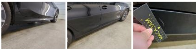
Door FR, Scratch(es), Repair and paint (complete)
