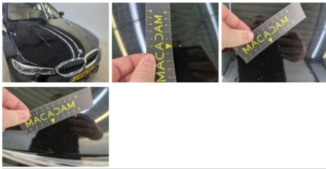
Bumper F, Scratch(es), Repair and paint (complete)
