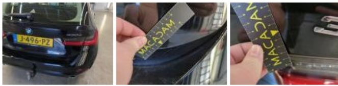
Rear spoiler, Scratch(es), Repair and paint (complete)
