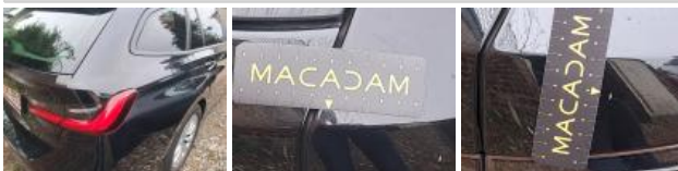
Wing RR, Dent(s), Paintless dent repair
