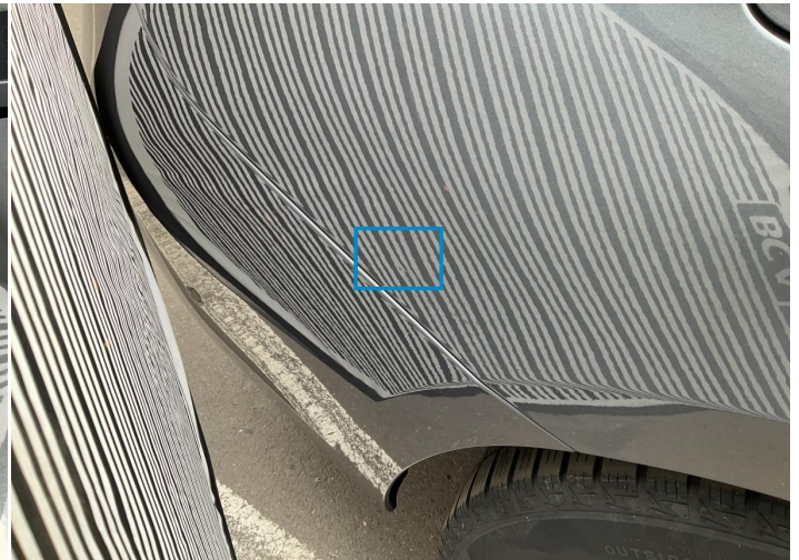
8. Side Panel / Back Right Bodywork / Dent / Dent -
