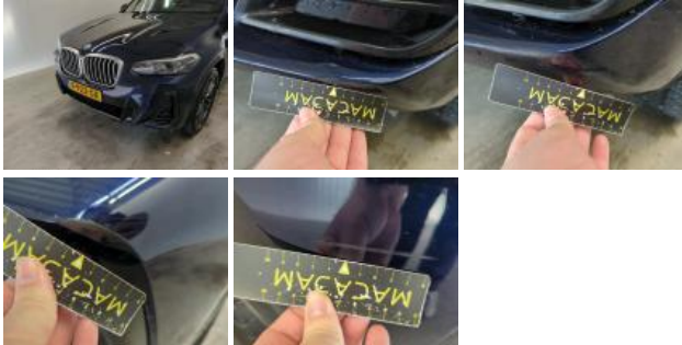
Bumper moulding FL, Scratch(es), Replace and paint
