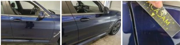
Wing RR, Scratch(es), Repair and paint (complete)
