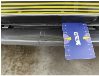
Bumper Front // Repair & Painting-dent
