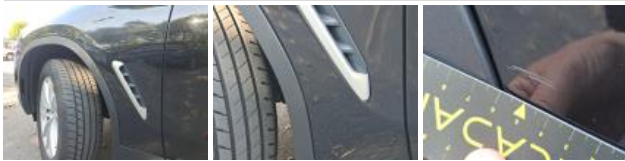
Door trim FL, Scratch(es), Spot repair
