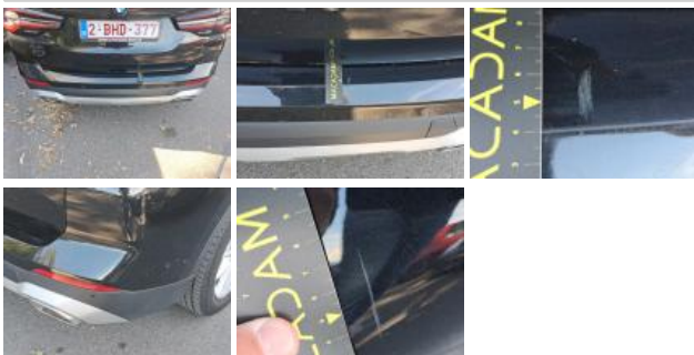
Bodywork, Paint measurement, Acceptable
