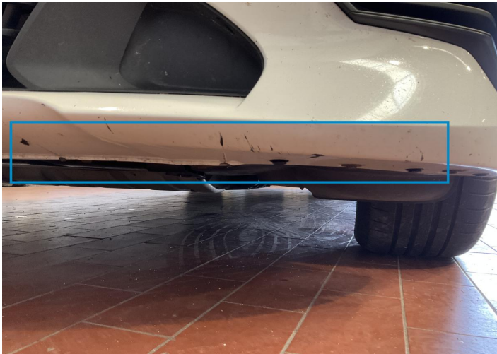
1. Bumper / Front Paint / Scratch / Scuff -
